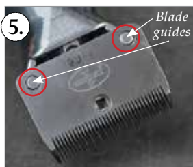
5. Place the bottom blade over the blade guides.
