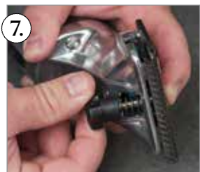
7. Thread tension nut/spring (A) onto tension bolt (B). Hand tighten until spring is fully compressed. Then untighten 2 full turns.
