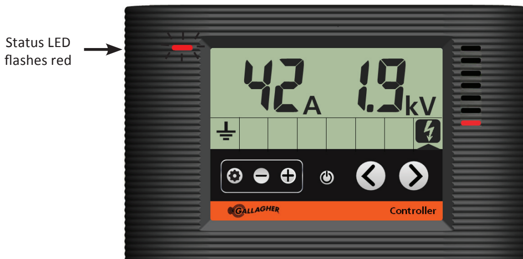
Controller showing the energizer in output alarm
