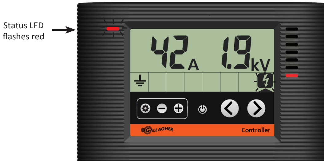
Controller showing the energizer in current alarm
