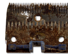
Example of severe rust
