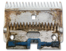
Example of dirty blades/light rust
