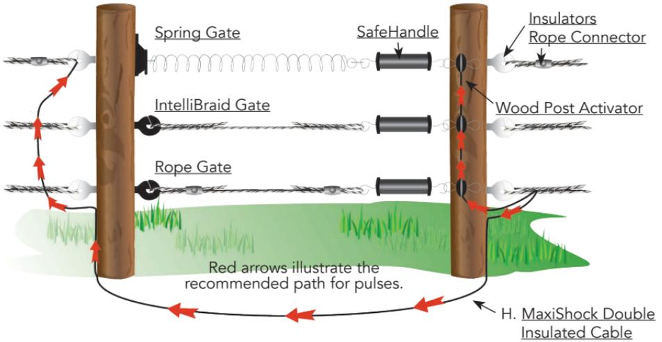
Don't rely on the gate to carry the power to the next fence. Instead, run insulated wire under gate openings to electrically connect fences on each side.
