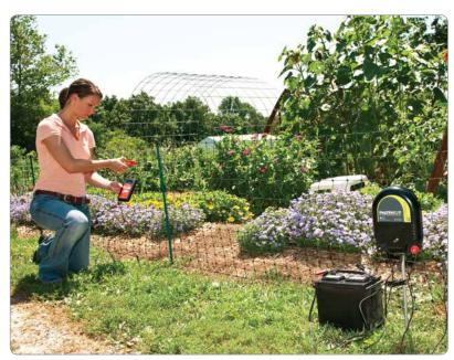
After turning on the energizer, test the fence with a voltmeter. Voltage should be at least 3000v.
