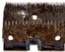
Example of rusty blades
