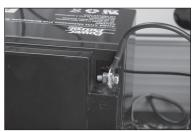
4. Unscrew the bolt of the black "-" battery terminal. Placement of bolt and wires as follows: bolt. washer, terminal, black wire, lock washer, nut (as shown). Tighten until wires are firmly held.
