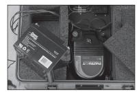
2. Lift the battery out of the foam pocket and set on the energizer case (as shown).
