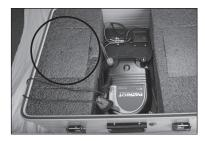
1. Looking at the inside of the PRS unit as in the picture, remove the left foam battery cover and set aside.
