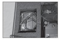
5. Place battery back into the foam pocket. The wires should be on top of the battery.
