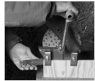
10. After kernels are gone, sheller pushes cob, out the back end so it doesn't fall into the shelled corn.
