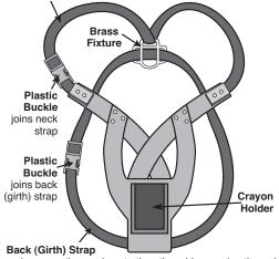
makes a continuous loop to the other side, passing through double loop of brass fixture on top of ram's shoulders
