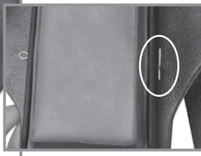
4. Metal Cotter Pin - Take the cotter pin and push all the way through the middle holes of the harness. Once the cotter pin is pushed through all the way bend back the ends flush with the crayon.
