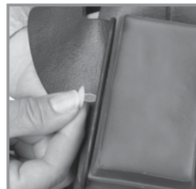
5. Plastic Pins (optional) - Use instead of the cotter pin. Push pins in holes on each side of harness.
