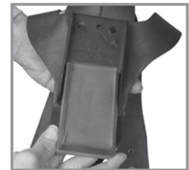
4. Slide the crayon into the harness by inserting the narrow end first.
