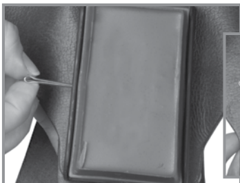
4. Metal Cotter Pin - Take the cotter pin and push all the way through the middle holes of the harness. Once the cotter pin is pushed through all the way bend back the ends flush with the crayon.
