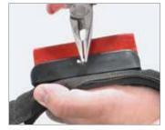
5b. Once the cotter pin is pushed through all the way bend back the ends flush with the crayon.
