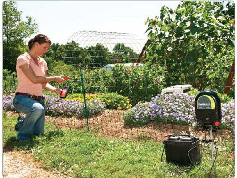
After turning on the energizer, test the fence with a voltmeter. Voltage should be at least 3000v.
