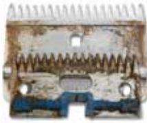
Example of dirty blades/light rust
