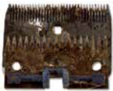
Example of severe rust
