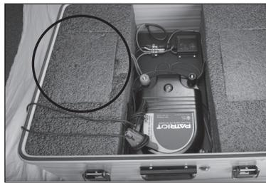
1. Looking at the inside of the PRS unit as in the picture, remove the left foam battery cover and set aside.
