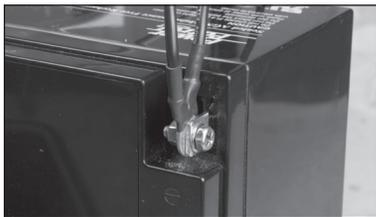
9. Unscrew the bolt from the "-" terminal and bolt in black "-" wires. Place battery back into the foam pocket.
