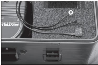
7. Lift the right battery out of the foam pocket and set on the energizer case. In the right pocket are 3 wires, 1 is red "+" and 2 are black "-".
