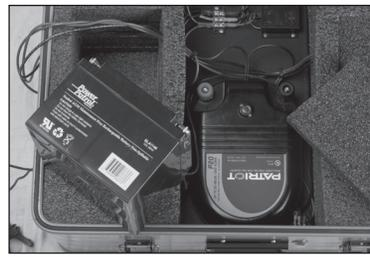
2. Lift the battery out of the foam pocket and set on the energizer case (as shown).
