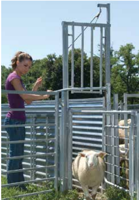
Sorting sheep with less effort. With her left hand, Kylie lifts a guillotine gate to allow sheep to exit. With her right hand she operates a two-way sort gate. Chute has both 36" and 45" tall panels.
