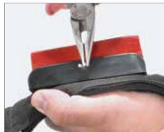
5b. Once the coter pin is pushed through all the way bend back the ends flush with the crayon.
