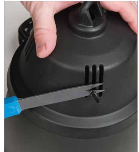
3. Cut/remove cable ties (they are not heat resistant).
