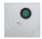
6. Place seal (B) over the threaded bolt (A). Thread nut (I) onto bolt (A) and tighten.
