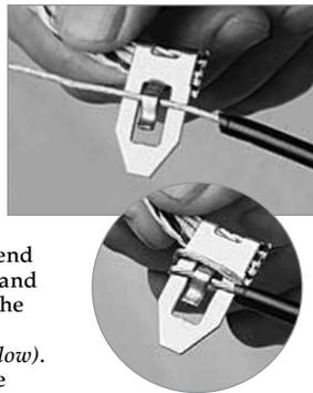
**Note:** Remember that with a net fence, the metal clip at the end of your fence DOES NOT connect back to the metal clip at the beginning of your net. Test the end of the fence ensuring adequate voltage.
