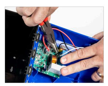
Disconnect any wires connected to the circuit board. There will be two from the transformer and possibly two from the external charging port.
