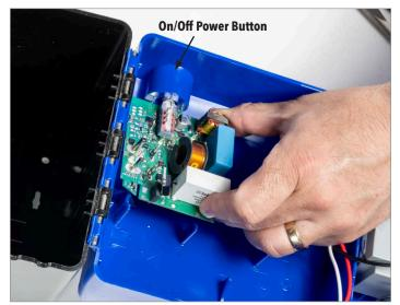
Remove old board by lifting the rear and pulling away from power button. Button will pop loose.
