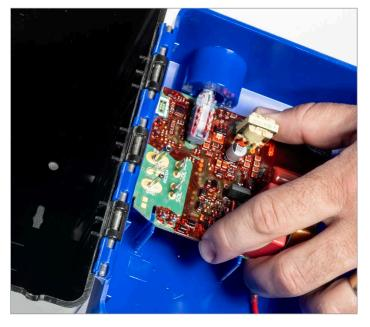
5. Insert new board and replace button. Press button in place as if you were turning on the energizer. Make sure button is in off position (sticking out).
