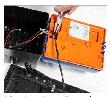
1. Open the energizer case. Using needle nose pliers, remove the solar panel and battery connections from the circuit board.
