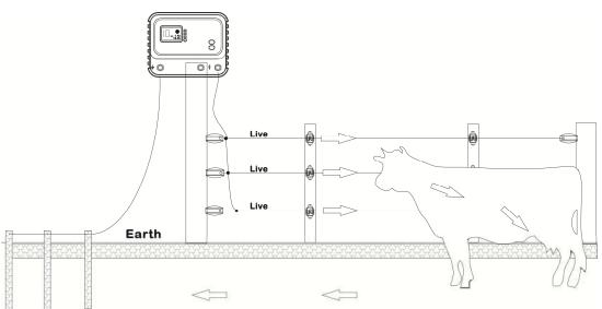
Pos./Neg. system: Where soils are not conductive e.g. dry, sandy, pumice soils as well as frozen soils or snow conditions, where an earth-return wire should be used in conjunction with the ground system – as per diagram. When the animal touches both a positive and a grounded wire, the animal will receive a shock.
