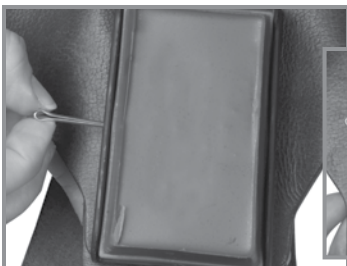
4. Metal Coter Pin - Take the coter pin and push all the way through the middle holes of the harness. Once the coter pin is pushed through all the way bend back the ends flush with the crayon.
