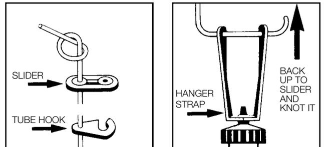
For the most efficient operation, it is necessary to suspend the Waterers above the height of the backs of the birds. With large birds and Layers the Waterers should be set at about their eye level.
