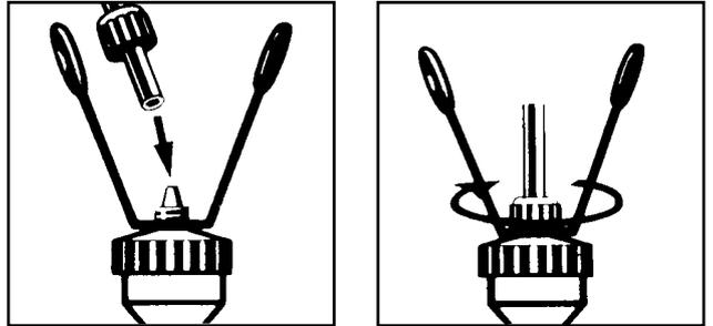
Place a nut, thread outwards, onto the end of the tube. Push Hanger Strap over filter top. Push the tube onto the tapered end of the filter top as far as it will go. Tighten the nut firmly. Repeat at the Saddle Connector end.
