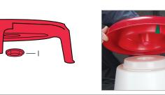
6. Set the base (H) onto the bucket (C).
