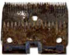
Example of severe rust
