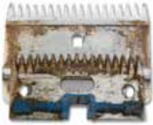
Example of dirty blades/light rust
