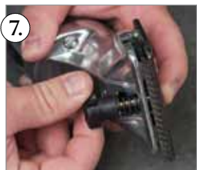
7. Thread tension nut/spring (A) onto tension bolt (B). Hand tighten until spring is fully compressed. Then untighten 2 full turns.
