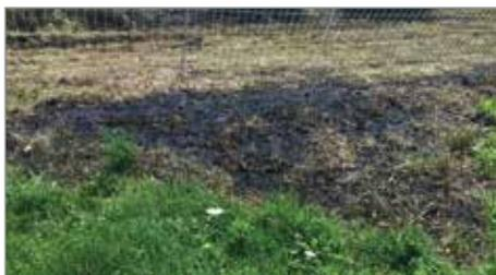
The lowest electrified strand (conductor) of the netting was in contact with combustible vegetation. The "continuous current" from this particular energizer combined with the vegetation to ignite a serious fire.
