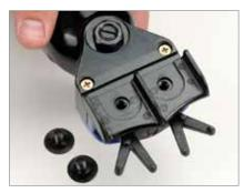
2. Place flat side of comb lifter onto shear head. The pointed side of the comb lifter should face the front of the shear head.
