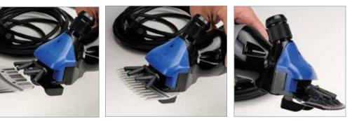
4. Insert comb between comb lifter and shear head. Apply comb and cutter per **"Tips to fit comb & cutter to shear head instructions."**
