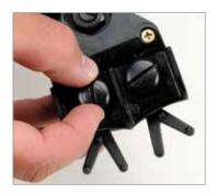
3. Reinsert screws through the comb lifter and into shear head.
