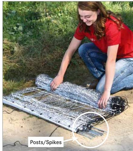
**Step 2.** Lay the folds of net neatly on the ground. Starting at the end opposite the posts, roll the folded net toward the posts. When this is done, use the exposed end-post tie strings to secure it as a roll.
