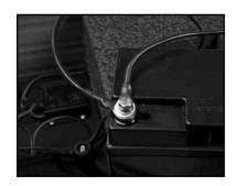
9. Unscrew the bolt from the "-" terminal and bolt in black "-" wires.
