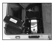
2. Lift the battery out of the foam pocket and set on the energizer case as shown. In the left pocket are 3 wires, 2 are red "+" and one is black "-".
