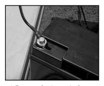
4. Remove plastic terminal ccover and unscrew the bolt from the black "-" terminal. With washers still on the bolt, attach the black "-" wire to the "-" terminal.
