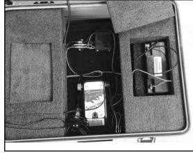
10. Place battery back into the foam pocket. The wires should be on top of the battery. Replace foam lid.
