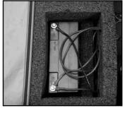
5. Place battery back into the foam pocket. The wires should be on top of the battery.
