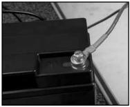
8. Unscrew the bolt from the red "+" terminal of the battery. Remove red tape from red "+" wire and bolt to the terminal, use same method as step 3.
