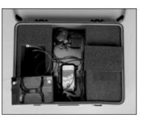
2. Lift the battery out of the foam pocket and set on the energizer case as shown. In the left pocket are 3 wires, 2 are red "+" and one is black "-".
