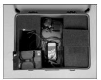
1. Looking at the inside of the PRS unit as in the picture, remove the left foam battery cover and set aside.
