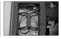
5. Place battery back into the foam pocket. Do not set battery on the wires, the wires should be on top of the battery.
