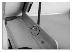
2. There are two brackets that are attached to the energizer case. Remove the wing nuts that are attached to these brackets (circled in photo). Attach both drop down supports to the brackets on the case with the wing nut and bolt. Your energizer is ready to be used.
