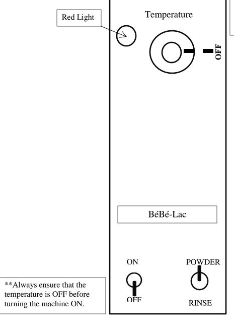
\*\*Always ensure that the temperature is OFF before turning the machine ON.
