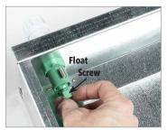
5. Turn adjustment screw to adjust water level.
