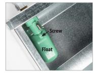
6. Top view of float. Adjust screw from top of float.
