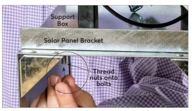
2. The support box is pre-drilled for the solar panel brackets. Insert the brackets into the top of the case and thread nuts onto bolts.
