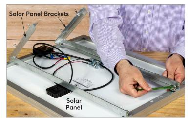
1. Attach the solar panel brackets to the back of the solar panel via bolts. Tighten with wrench.
