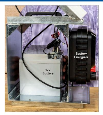
4. Set the battery inside the support box. Attach the solar panel leads to the battery terminals, "+" to "+" and "-" to "-". Connect the energizer's battery adapter to the panel clamps, red to positive and black to negative.
