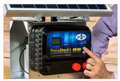
5. Check the front panel to see if the energizer has power, do not touch the terminals. Disconnect power until you are ready to fence. When the fence is ready to be energized: Connect the energizer to the fence, ground rod and finally the battery. For maximum sunlight, orient the unit so the panel faces south.
