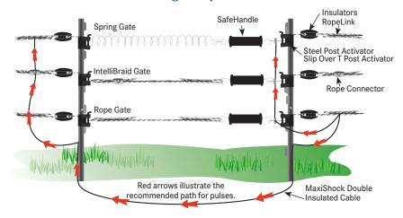
Don't rely on the gate to carry the power to the next fence. Instead, run insulated wire under gate openings to electrically connect fences on each side.
