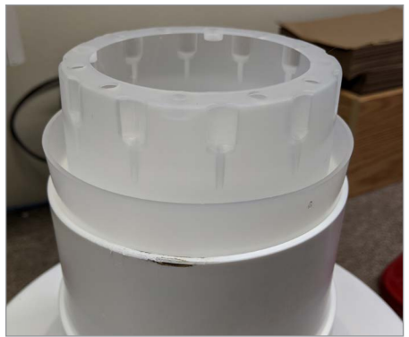
6. Float housing pressed down into the water tank. This step is usually missed and will result in water inside the trough, but not much.
