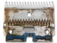
Example of dirty blades/light rust
