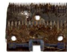
Example of severe rust
