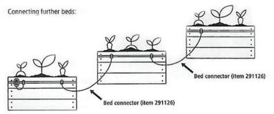
please always note the maximum permissible fence length of 30 m. Beyond this length, the effect of the fence can be reduced and the battery service life can also be significantly shortened.
