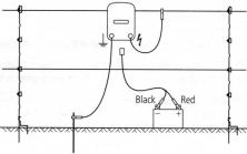
*Note:* If required, this energizer can be used as part of a solar installation, by connecting it to a battery and solar panel(s). For information about solar installations, refer to the product's website (see packaging for details).
