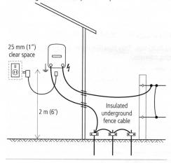
*Note:* If the energizer is being installed inside, it may be powered by a battery instead of the mains/line power supply, if required.
