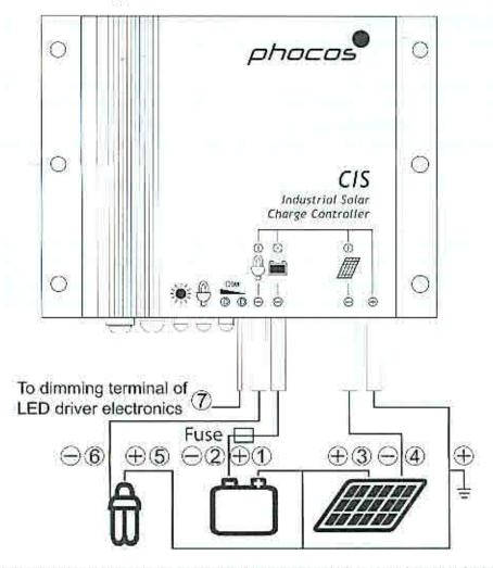
IMPORTANT: Connect wires in the order indicated 1 2 3 4 5 6 7 to avoid installation faults!
