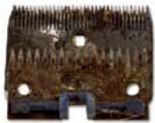
Example of severe rust
